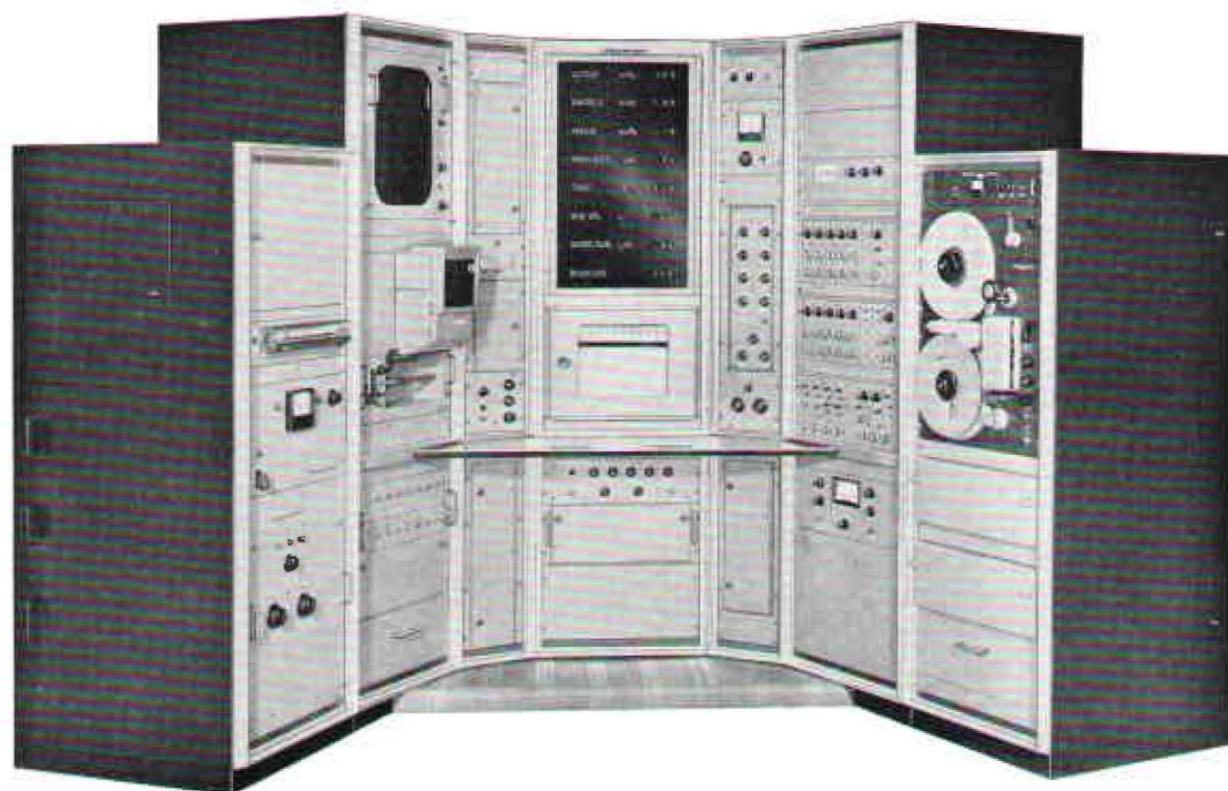
One of four monitoring consoles, engineered and built for NIH by Sanborn, is a complex but thoroughly integrated system of instruments. Clearly visible are such pieces of Sanborn equipment as an 8-channel oscilloscope, photographic oscillograph, 8-channel digital display, preamplifiers, and magnetic tape recorder.
